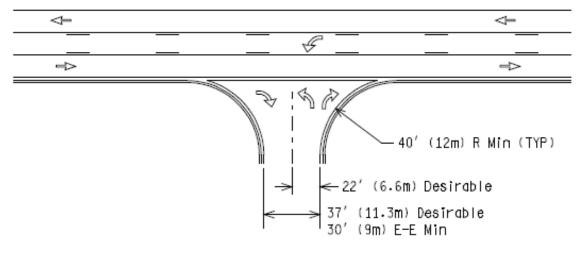
(For Three Lanes, Width Should Be 39' (11.7m) Min)
